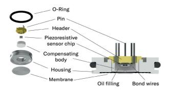
Figure 2: Construction of an insulated, oil-filled
