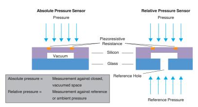
Figure 1: Structure of a piezoresistive sensor chip.
