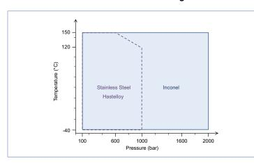
KELLER 6LHP series high-pressure transducers are available with various material options. Stainless steel, Hastelloy C-276, Inconel 718 or titanium can be selected (see "Mechanical data") in line with requirements.
